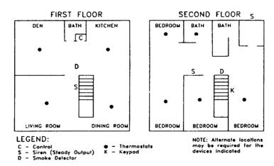
NOTE: Installation of fire detection equipment in all rooms and areas of the household is suggested for early warning fire detection. A smoke detector should be installed on each level and in each separate sleeping area (the vicinity of, but outside of the bedroom), with heat or smoke detectors in living rooms, dining rooms, bedrooms, kitchens, hallways, attics, furnace rooms, closets, utility and storage rooms, basements, and attached garages.
