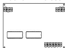
The PC5132 Wireless Receiver module can be used to connect up to 32 wireless devices. All devices are spread spectrum, 900 MHz, fully supervised and use standard 'AAA' or 'AA' alkaline batteries (See Section 5.27 "Wireless Expansion"). (See *PC5132 Installation Manual*.)
