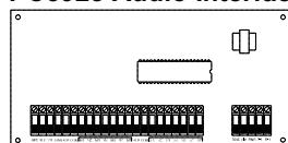
The PC5928 Audio Interface module is a simple way to incorporate paging, intercom, baby listen-in and door answer to the PC5101 control panel. The module also has built-in two-way voice capability for central station (See Section 5.30 "Audio Interface Module").
