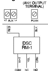
Each PGM output is an open collector switch to ground. That is, when the PGM output is activated by the panel the terminal will switch to ground.
