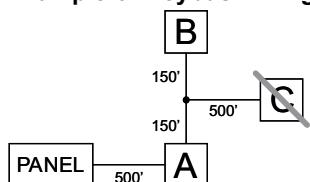
NOTE: Module (A) is wired correctly as it is within 1,000'/305m of the panel, in wire distance.
