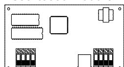
This Escort5580 module will turn any touch tone phone into a fully functional keypad. The module also includes a built-in interface to control up to 32 line carrier type devices for lighting and temperature control (See Section 5.28 "Escort5580 Module"). (See Escort5580 Installation Manual.)
