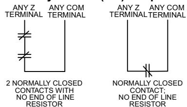
To enable normally closed loops, programming section [013], option [1] must be ON.
