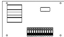
The PC5204 can provide up to 1 Amp of additional power for modules or devices connected to the control panel. The module requires a 16.5 volt AC 40 VA transformer and 4 AH battery. In addition, the module provides 4 programmable high current voltage outputs. Each output is individually programmable with 19 PGM output options available (See Section 5.10 "PGM Outputs"). (See PC5204 Installation Instructions Sheet.)
