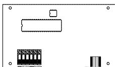
This PC5400 Printer Module will allow the panel to print out all events that occur on the system to any serial printer. All events will be printed with the Partition, time, date and the event that occurred (See Section 5.29 "On-site Printer").
