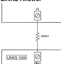
If the LINKS1000 cellular communicator is being used a zone may be configured for LINKS Answer to allow downloading to be performed in the event of phone line failure.
