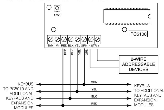
The PC5100 will allow addressable multiplex loop devices to be added to the system. These devices use a 2-wire connection for power and to communicate with the control panel. This, in combination with low power device, simplifies wiring and reduces device count for fast and efficient installation.
