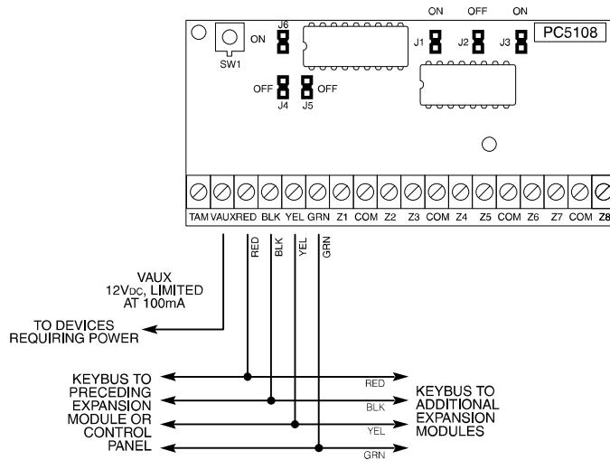
In this diagram the jumpers settings shown indicate the first group of four zones of the expander will be zones 9 to 12 and the second group of 4 zones will be 13 to 16.
