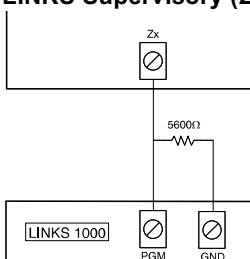
When using the LINKS1000 cellular communicator, any main board zone may be configured for LINKS Supervision. Program this zone as zone type [09], 24 Hour Supervisory in section [001].
