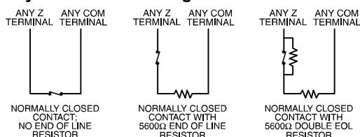
Zones may be programmed to be used as keystwitch arming zones and must be wired according to the following diagrams:
