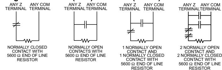
To enable panel detection of single end of line resistors, programming section [013], options [1] and [2] must be OFF.
