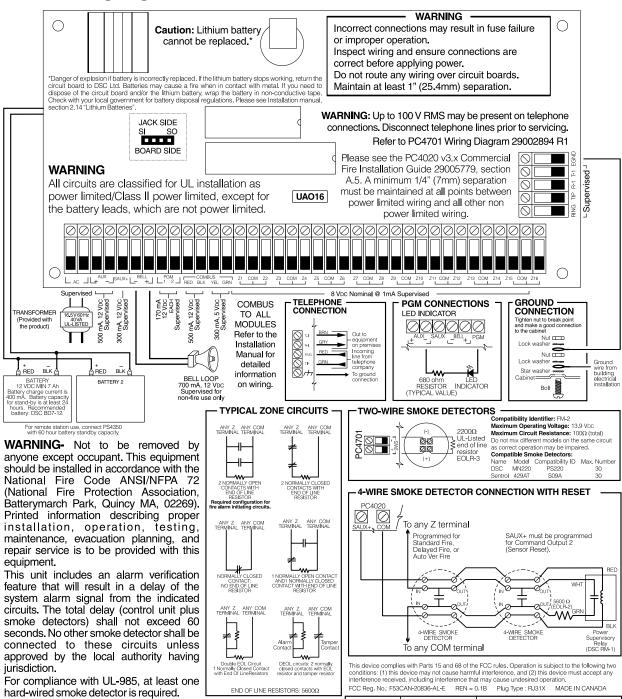
Refer to the Installation Manual P/N 29005774, Instruction Manual P/N 29005777 and PC4020CF Commercial Fire Installation Guide P/N 29005779 for complete operating instructions. The PC4020 is UL-Listed for Inmitted energy installations per NEC Article 760. Recognized limited energy cable should be used. Observe NEC wiring requirements and local codes defined by the authority having jurisdiction.
