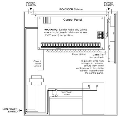
INSTALL BATTERY AND AC WIRING AS SHOWN ABOVE IMPORTANT: A minimum 1/4" (7mm) separation must be maintained at all points between battery/primary AC wiring and all other wiring connections.
