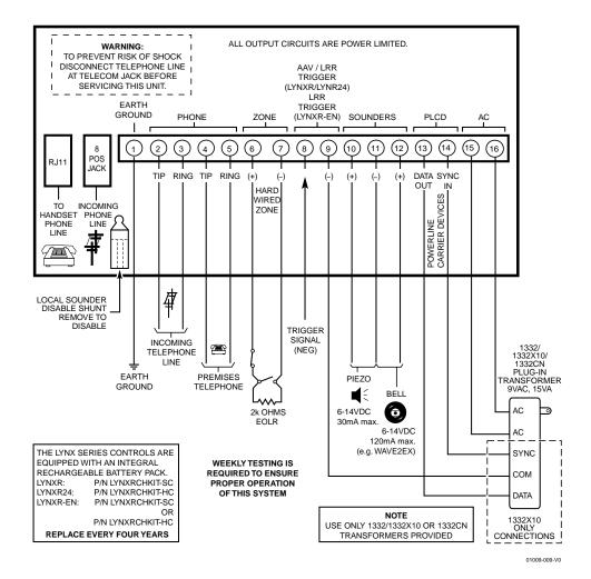
LYNX-R-SERIES WIRING CONNECTIONS
